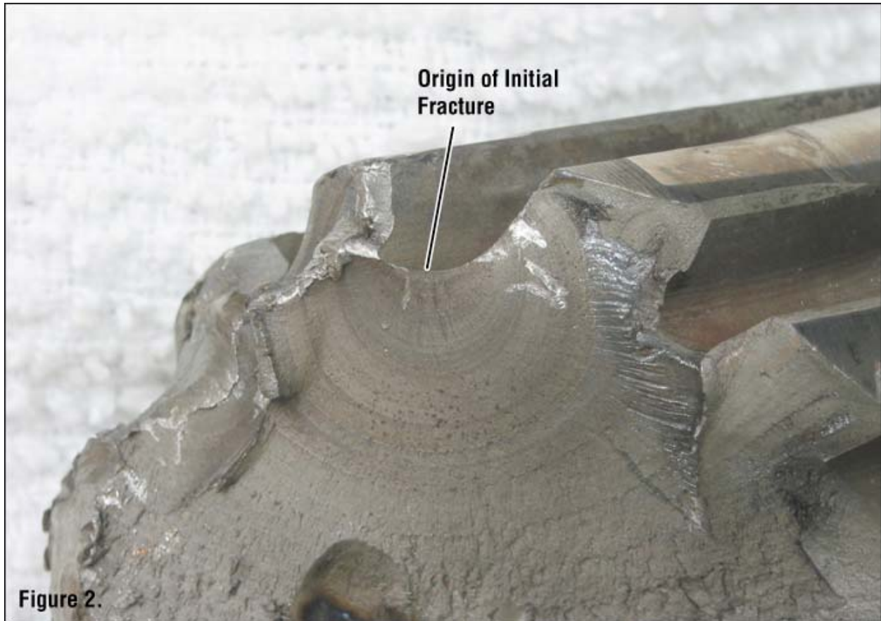
Figure 2. Rearward End of 45 Degree Fracture: A close-up of the rearward end of the fracture—origin of the initial fracture. The fracture began at the bottom of a spline root and progressed slowly across the diameter of the shaft at a 45° angle. The crack grew until the cross section was reduced to a threshold where the shaft could no longer transfer torque and the final fracture occurred.
