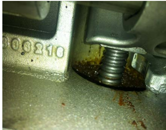
Inspect XY shifter for sludge build up and corrosion around the ballscrew to motor connection.
