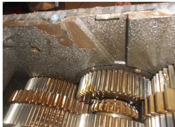
Contamination caused by engine coolant entering the transmission.
